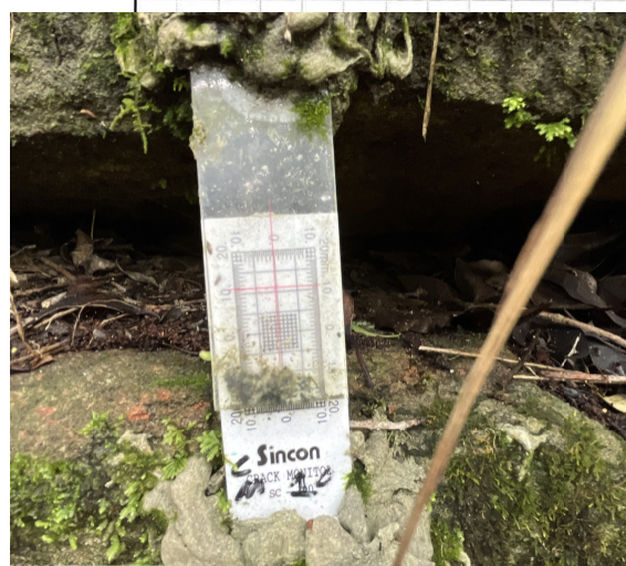
crack monitor on "new" wall
