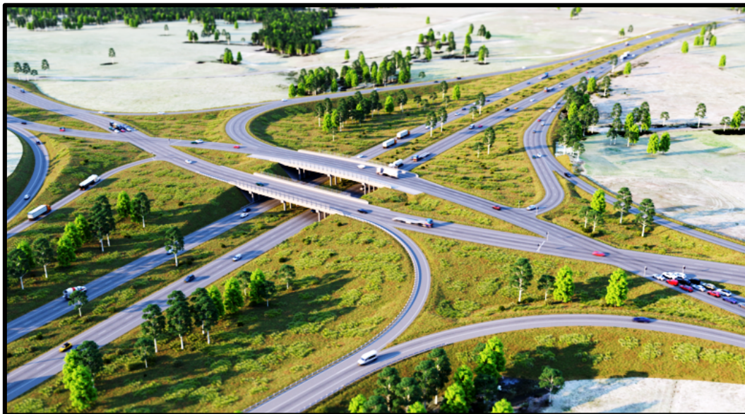
Diverging Diamond Interchange design by TfNSW
